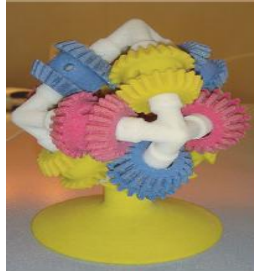
Figure 11.1 (a) Color output from a 3D printer: all the gears and rods in this model were ‘printed’ in one pass from bottom to top, and when one gear is turned, the others turn too.
